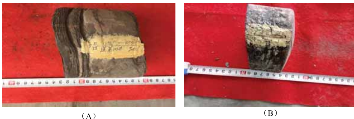
FIGURE 2 Cores of mudstone and oil sandstone samples from Shaximiao Formation in well Qinglin-1 (A) mudstone; (B) oil sandstone
