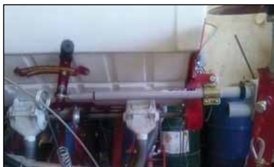
FIGURE 1 Implemented flow rate control mechanism
