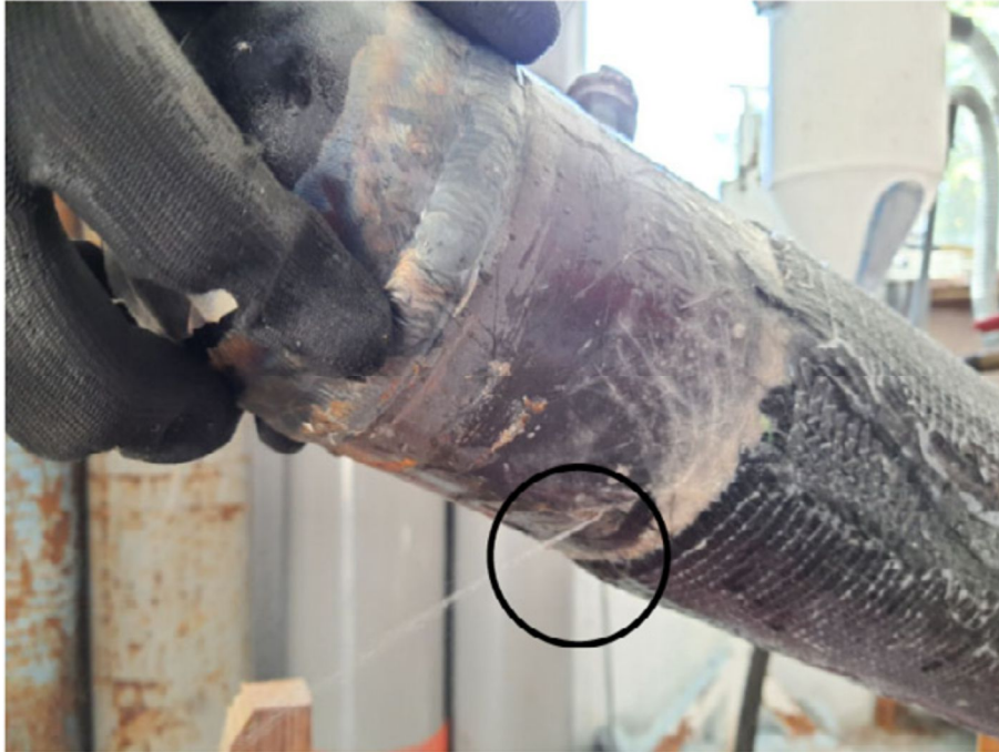
Fig. 21. Detail of the test fluid bursting on the edge of the composite patch.
