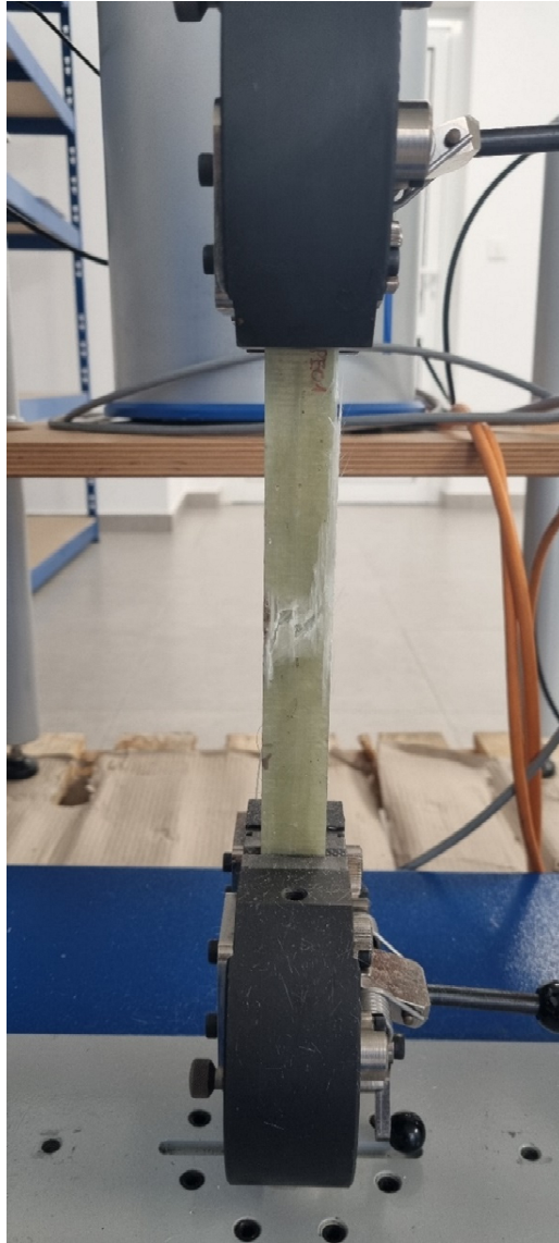
Figure I.7 Coupon on completion of the tensile test
