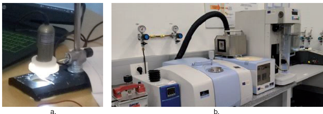
Figure 1 Instruments for the analysis performing: a. digital microscope; b. FTIR spectrophotometer with TG-IR interface
