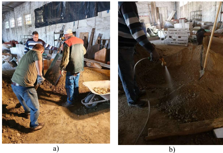
Fig. 2. Preparing material: a) sieving, b) adding water
