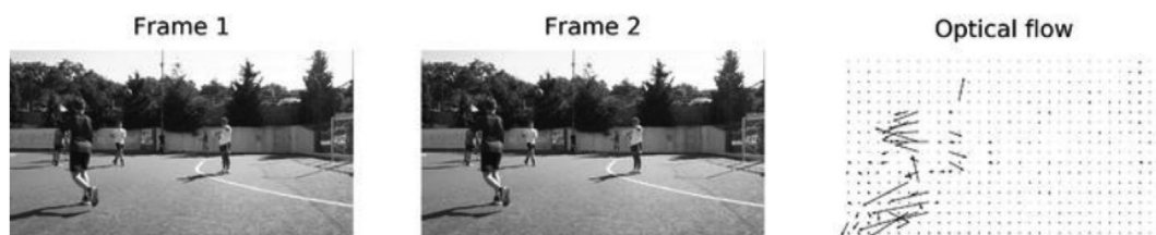
Figure 5. Example of two adjacent frames in a video and the corresponding Optical Flow field [16].
