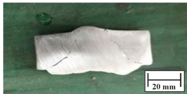
Figure 11. Specimen image after iron (III) chloride solution treatment for 72 hours at 40 °C
