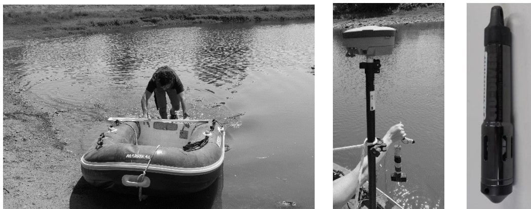
Figure 5. Equipment used for the bathymetry measurement (from left to right): Inflatable boat, Topcon positioning system HiPer V and CTD – diver [7]
