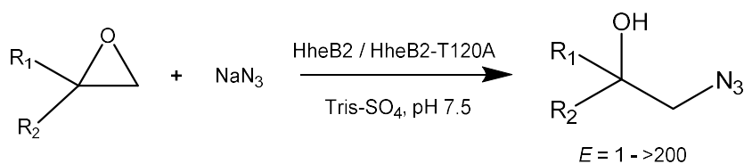
Figure 1. Nucleophilic ring-opening of epoxides catalysed by HheB2 from Mycobacterium sp. GP1 and mutant HheB2-T120A
