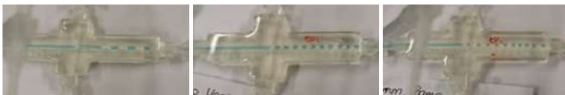
Figure 1. Droplet size is controlled by surface modification and changing the flow ratio of the two liquids in the droplet generator
