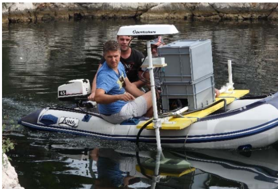
Figure 6: The MBES survey of the Lake Zmajevo oko.
