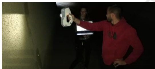
Figure 7: Scanning of test surface using Artec Eva.
