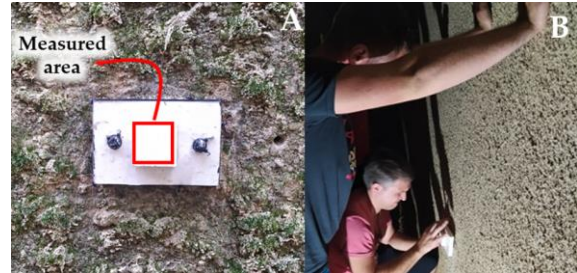
Figure 5: (A) Limestone PL measured with CMD; (B) installation of PL on the lateral sides of tunnel in no-light condition.
