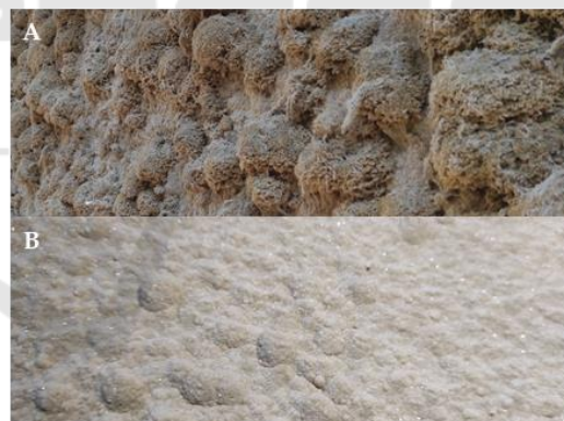
Figure 16: (A) Test surface with highest increment; (B) hard sedimented tufa inside the tunnel.
