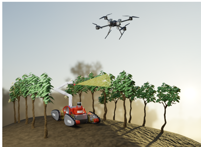
Figure 1. An artist's view of a heterogeneous robotic system for work in viticulture, consisting of a light autonomous aerial robot and an all-terrain mobile manipulator.
