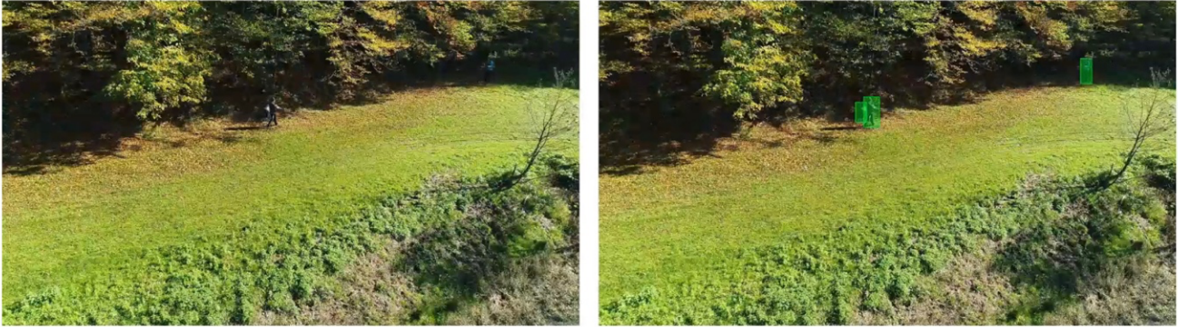
Fig. 1 – Aerial image, taken by a drone (left). Detection of persons (green bounding boxes) performed by YOLO v4 (right).
