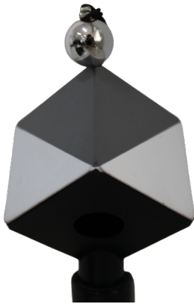
Fig. 2. SpyderCube used for illumination extraction
