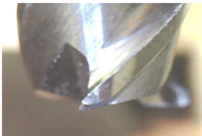
Figure 8. A worn tooth of the tool
