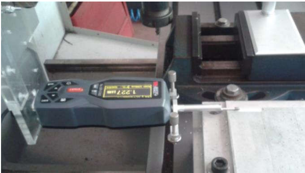
Figure 7. Measurements of the roughness parameters after the first milling pass
