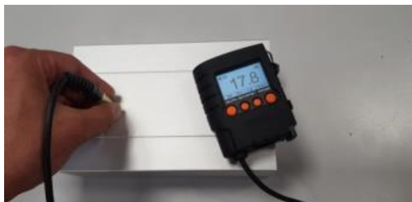
Figure 16. Eddy current height/width measuring gauge [21]
