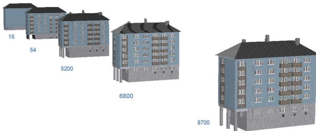
Figure 4.3. Representation of number of triangles in different LODs (URL 13)
