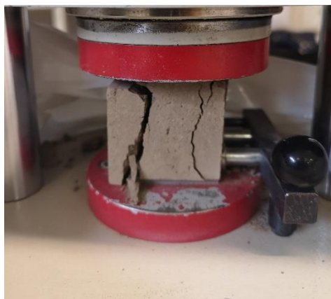
Figure 5. Testing compressive strength.
