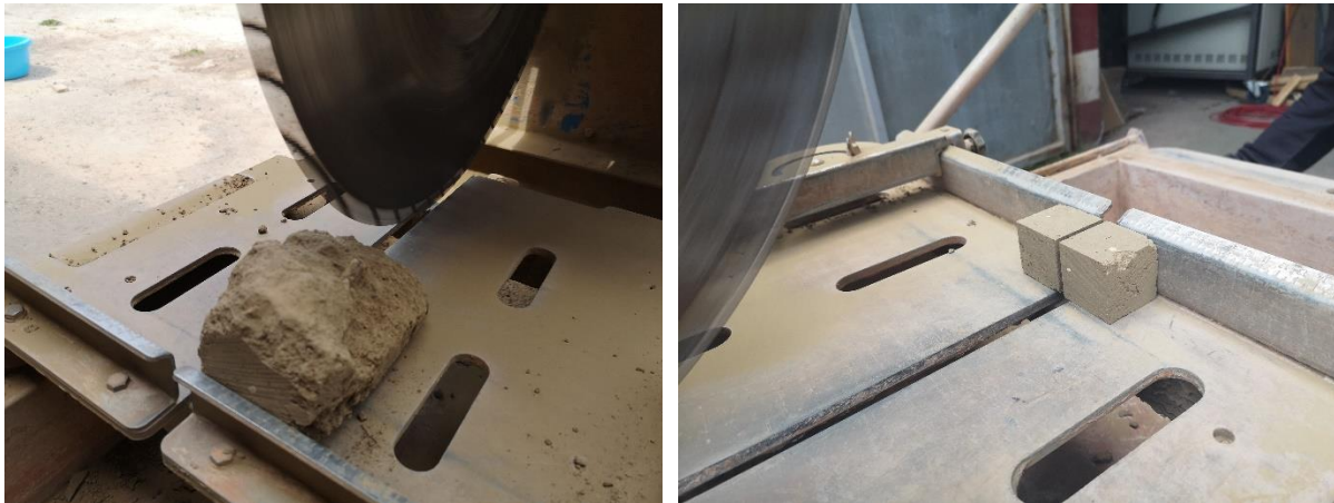
Figure 4. Cutting earth chunks into cubes for testing compressive strength.
