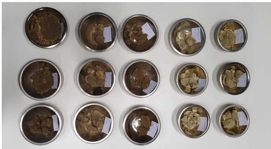
Figure 3. Samples for determining moisture content.
