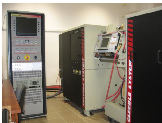
Figure 1: Gleeble 3500 thermo-mechanic physical simulator installing at the Department of Mechanical Technology at the University of Miskolc
