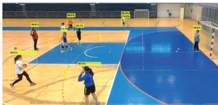
Figure 4. Player detections in handball scene with YOLOv3 (bounding boxes with confidences).
