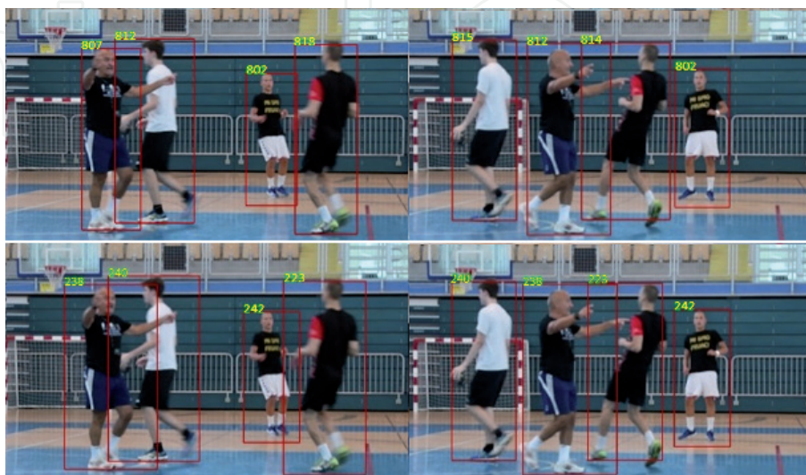
Figure 6. An example of tracking situation with occlusion. Top: Hungarian algorithm, bottom: Deep SORT. The left and right frames are 1 second apart.
