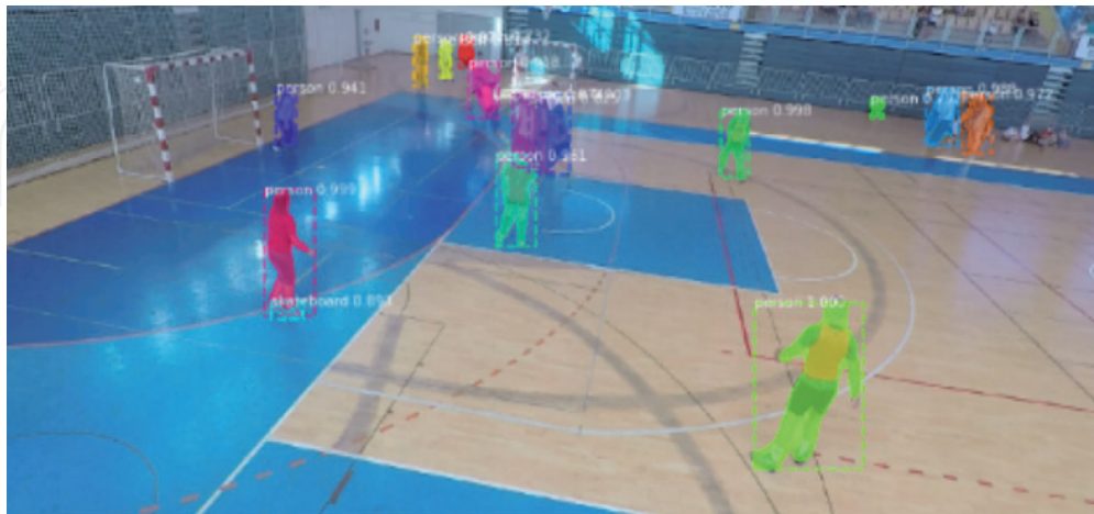
Figure 5. Player detections obtained with mask R-CNN in a handball scene (bounding boxes with segmentation mask and confidence value).
