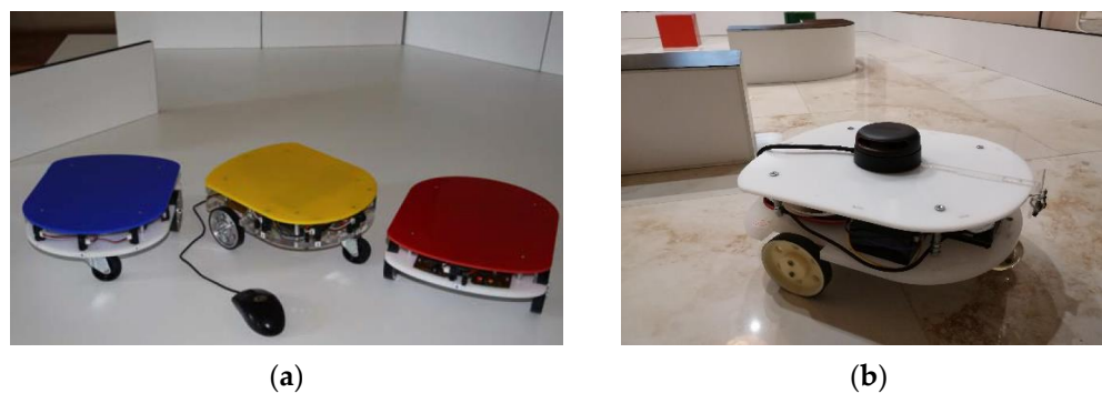
Figure 1. Mobile robots: (a) an older generation equipped with Infrared (IR) range sensors; (b) a newer generation equipped with laser range sensors.
