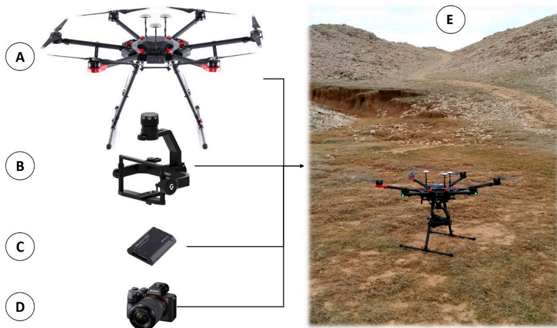
Figure 3. Different components functionally integrated into RAPS (A–D); application of developed RAPS for aerial survey of gully Santiš (E).
