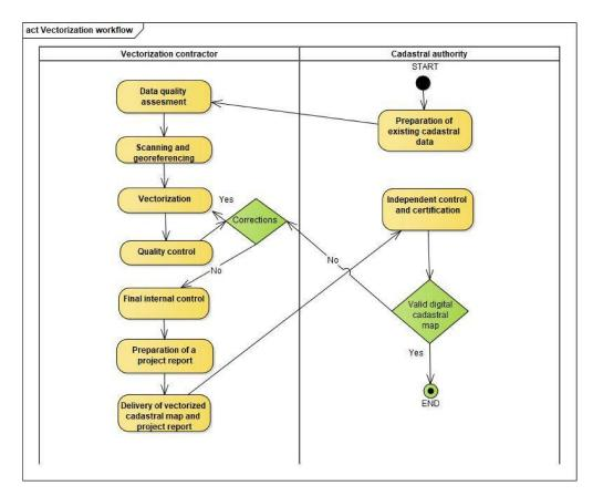
Figure 1. Vectorization flow diagram. Source: own compilation.
