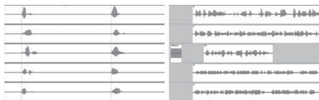
Fig. 4: Left: example of the DAW audio track arrangement in tests with logatomes with one referent and four distracting logatomes; right: example of the arrangement in tests with sentences for one reference speaker (middle row) and 4 distracting speakers
