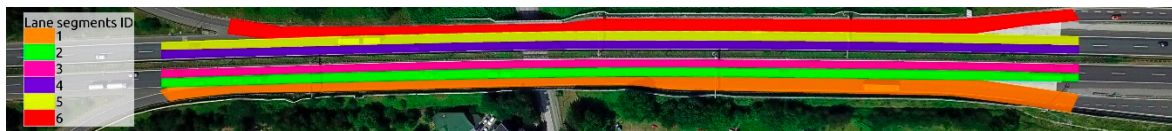
Figure 6. Marked lane segments of the observed area used for calculating segment-based traffic flow parameters.
