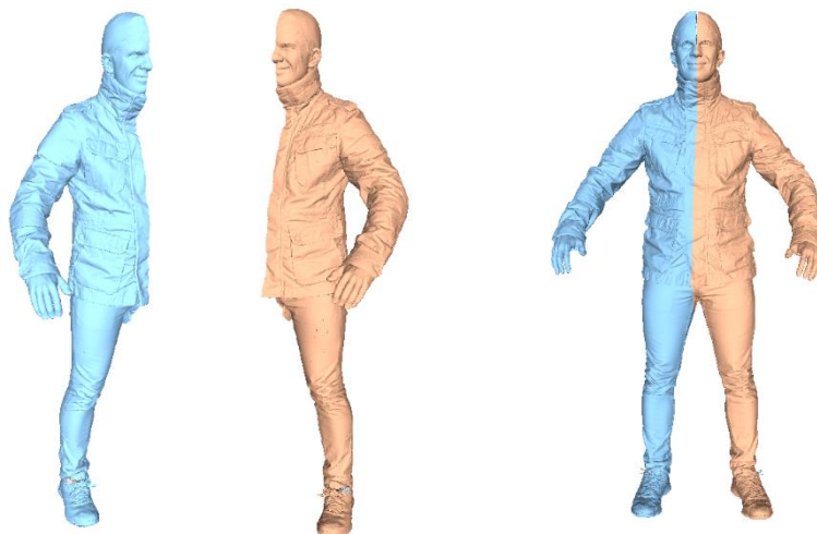
Figure 1: Example of partial registration of two point clouds.
