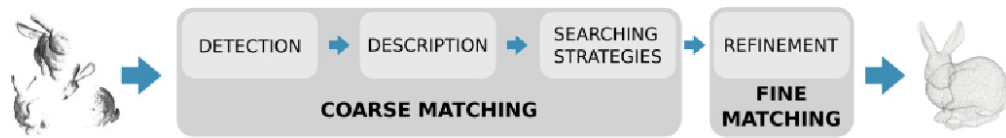
Figure 2: Pipeline of the detection-description-matching approach. Taken from [13].
