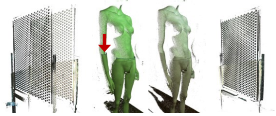
Figure 8. Point-cloud reconstructions: On the left are reconstructions using calibration data of Zhang's method when a single position of the board was selected as referenced. On the right are same reconstructions using calibration data from bundle adjustment.
