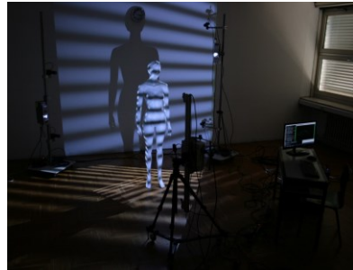
Figure 1. A 3D surface scanning system comprised of three projectors and six cameras
