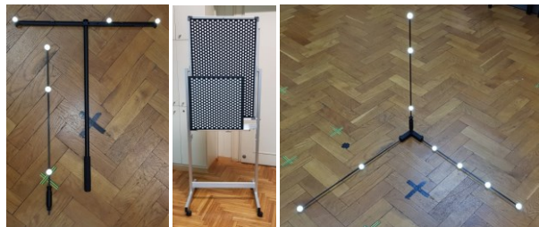
Figure 2. Various calibration objects: calibration wands (left), calibration boards (center), and a 3-axis spatial calibration object (right)
