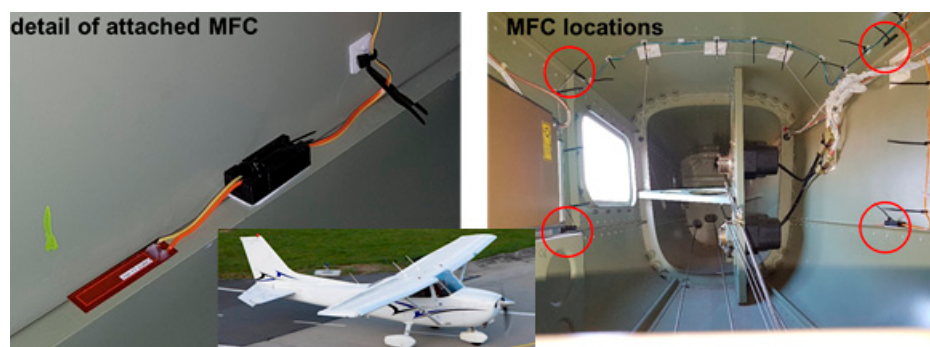
Figure 17. MFC patches embedded into the structure of a small civil aircraft [29]—reprinted by permission from Elsevier.
