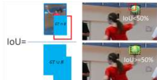
Fig. 2. Visual representation of intersection over union (IoU) criteria equal to or greater than 50% [21]
