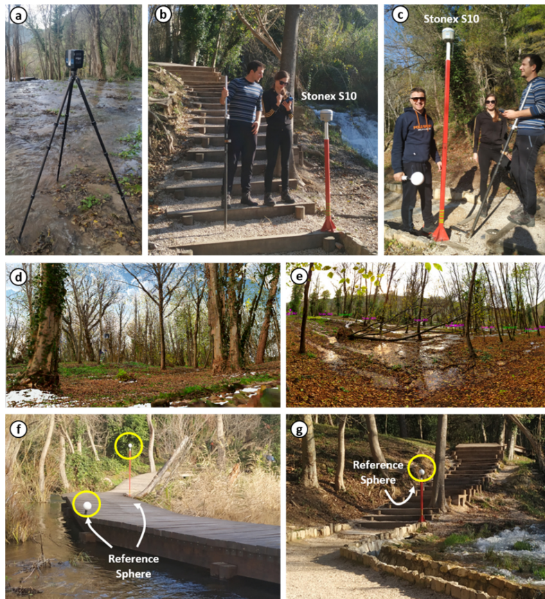
Figure 9. (a) Faro Focus M70 results on the test surface; (b,c) coordinate collection of the reference spheres using Stonex S10 (d,e) examples of a dense point cloud from selected scanning points; (f,g) examples of set reference spheres for dense point cloud orientation.
