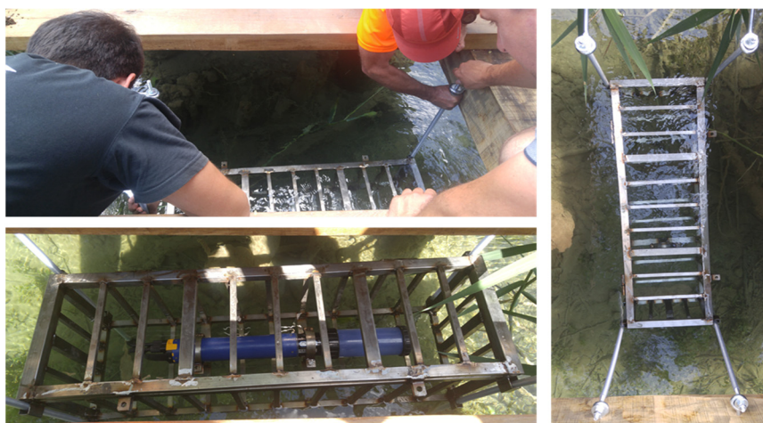
Figure 15. Placement of the probe in a metal non-oxidizing cage near the P3 location.
