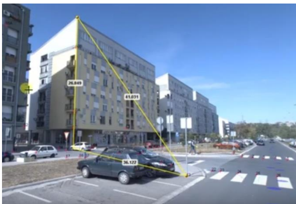
Figure 1: Checking the objects' dimensions after mapping
