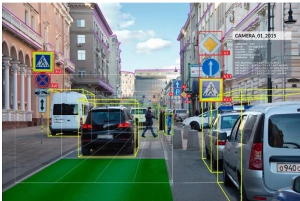
Figure 3: Feature identification and recognition by means of artificial intelligence
