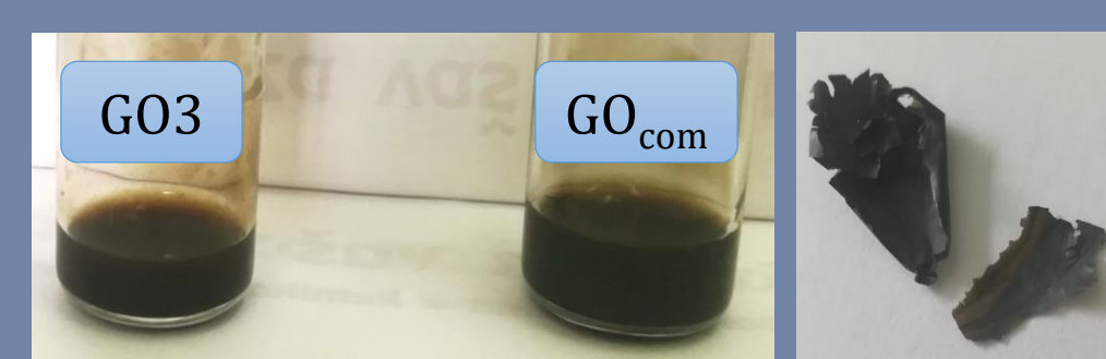
Figure 2. On the left is shown synthesized sample GO3 and commercial GO from Graphenea. Figure on the right represents dry GO3 (vacuum oven, 40 °C)
