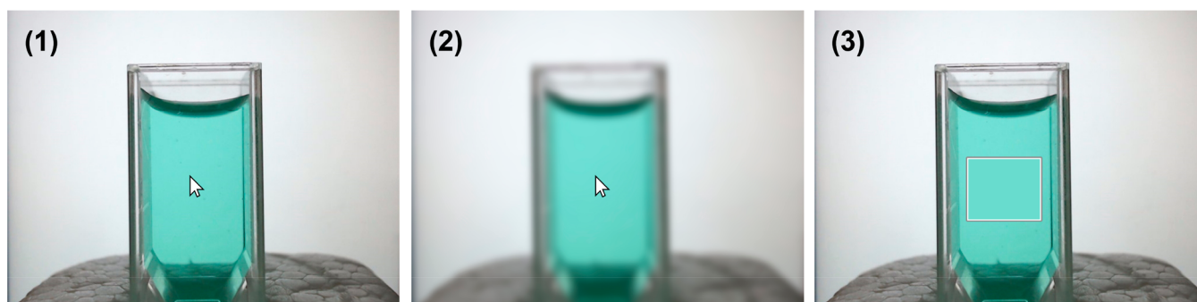
Figure 2. Graphical representation of the developed methods: (1) determination by pixel, (2) determination by pixel with Gaussian blur, and (3) average RGB.
