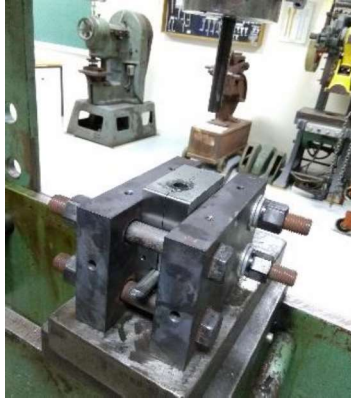
Fig. 2: ECAP tool utilized for severe plastic deformation
