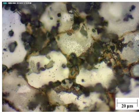
Fig. 5: Globular microstructure of the sample F with 500 x magnification
