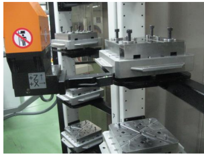
Figure 7 – Palette code reading in the pallet repository, using the manipulator
