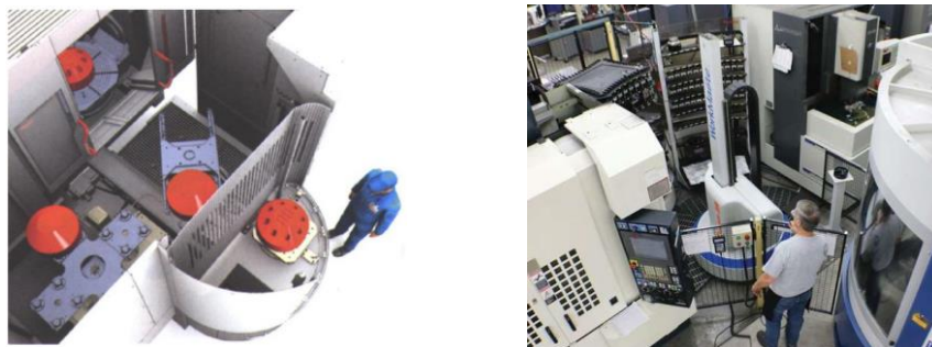
Figure 4 – a) Two-pallet manipulation table; b) Palletized FMS for changing pallets between multiple CNC machines and EDM machine
