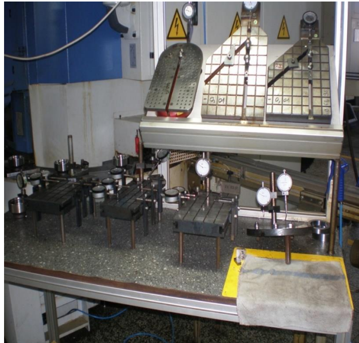
Figure 1. Contact measurement setup for bearing rings [1]
