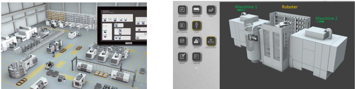
Figure 10 – The control system organizes, controls and visualizes production systems
