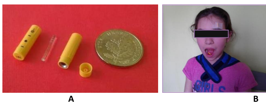
Figure 1. Picture of radiophotoluminescent (RPL) glass dosimeters GD-352M with and without shielding in relation to 5 lipa coin (A) and their position on the head, above the left eye and below the tongue (B)
