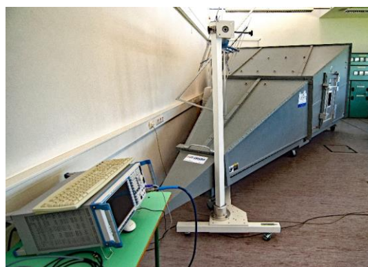
Figure 1. The GTEM cell used with a spectrum analyzer connected
