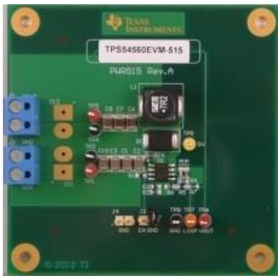
Figure 4. EUT (TPS54560EVM-515 Board)
