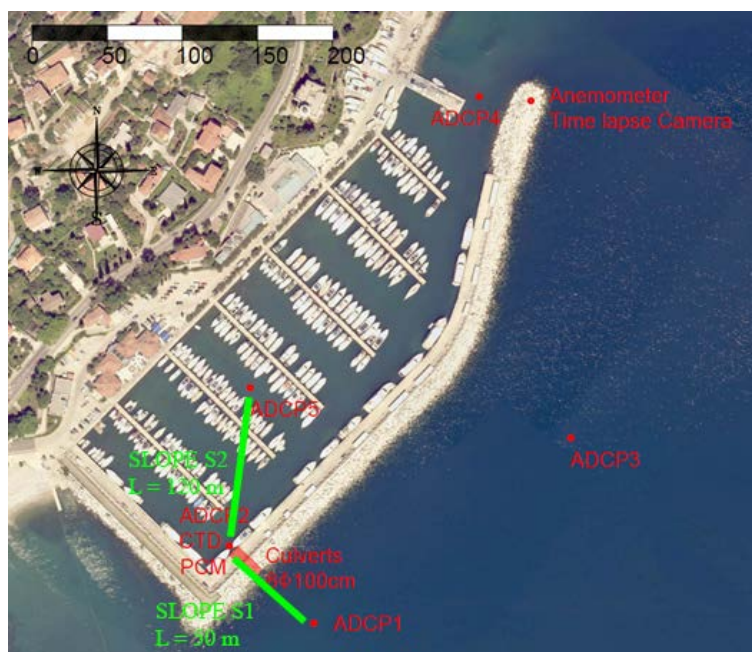
Figure 1. Plan view of the ACI marina Opatija with locations of measuring devices during the winter measuring period and sea surface slopes (S1 and S2) defined near the flushing culverts
