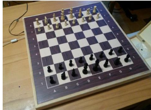
Figure 1. Digital chess board with: 64 Hall-effect sensors placed under each field, PC communication and power cables.
