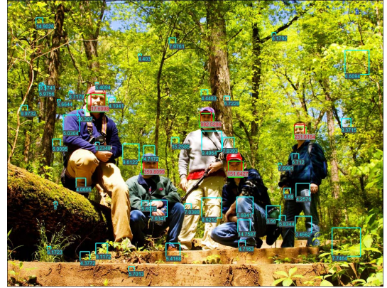
Figure 1. Example of the results of the NPD detector for the threshold \theta_{NPD} = 0 . The green squares denote ground truth, the red true positive, and the blue squares denote false positive. The ScoreNPD(I, S_i) is given at the bottom of each square.
