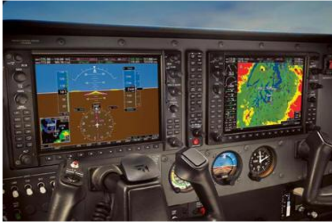
Figure 3. Example of glass cockpit [9]
