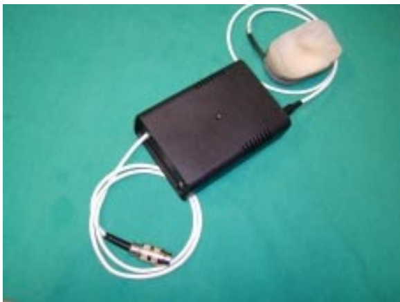
Figure 4. View of capacitive sensor and electronic part of force transducer
