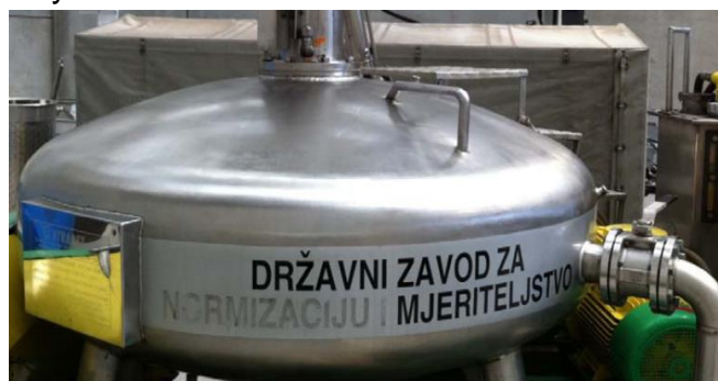
Figure. 3. Shows measurement etalon AM 1500 ET with capacity of 1500 litres [1, 5]
