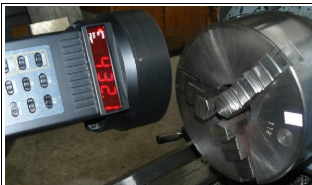
Fig. 3 Measurements done with stroboscope PCE-OM 15
