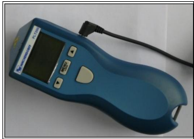
Fig. 4 Additional measurements were done with digital tachometer PCE 155
