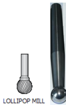
Fig. 5 Tool used in the proces is similar to lollipop mill and was made of carbide steel
