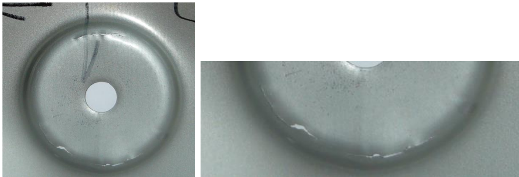
Fig. 9 Crack occurred in the rolling direction 0^\circ
