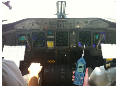
Fig. 6. Locating the audiometer in the Dash 8Q-400 cockpit space
