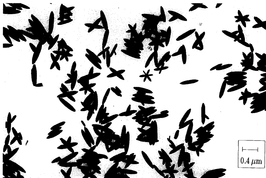
Fig. 3. TEM micrographs of sample S3. Needles, X- and Y-shaped \beta -FeOOH particles are visible.
