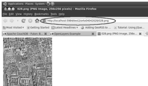
Figure 5 Accessing one tile via REST interface
