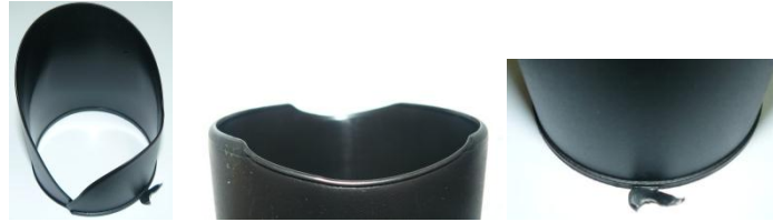
Fig. 5 Errors caused by wrong temperature parameters
