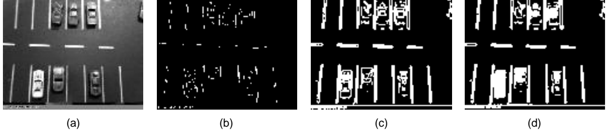
Fig. 4. Parking lot with six cars parked; (a) gray scaled image; (b) binary image after Sobel edge detection; (c) binary image dilated; (d) binary image after filling isolated regions with white pixels.
