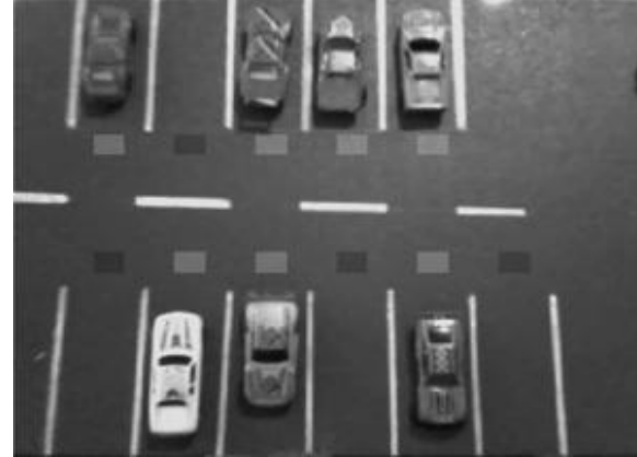
Fig 3. Parking lot model with indicators for free and occupied parking places.
