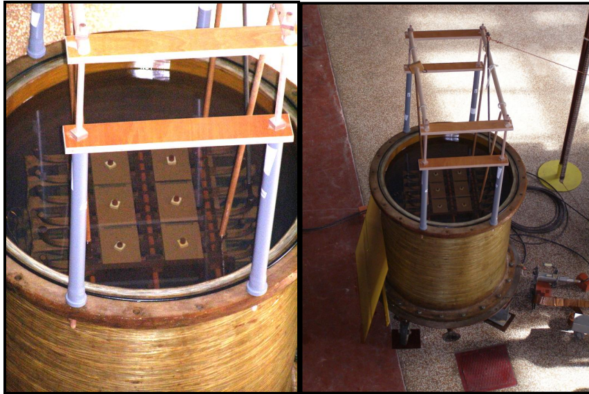
Figure 3: Models under testing (left: models under oil in the test vessel, right: test arrangement in HV laboratory)
